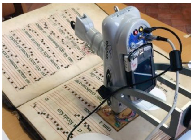
Figure 1. In-situ h-XRF analysis of the Codex Manizola 116C, f.13v. ©BPE and HERCULES Lab.
